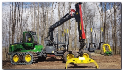
1. HAAS-OSA clamping bank for two different positions, second stake and headboard can be moved horizontally.
