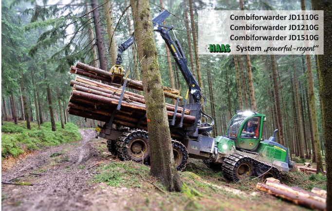
HAAS-ÖSA Clamping bank with extended movable rear for short logs.
