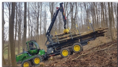
2. Stake cage with two stakes, second stakes horizontal extendable (assortment 2x3m).
