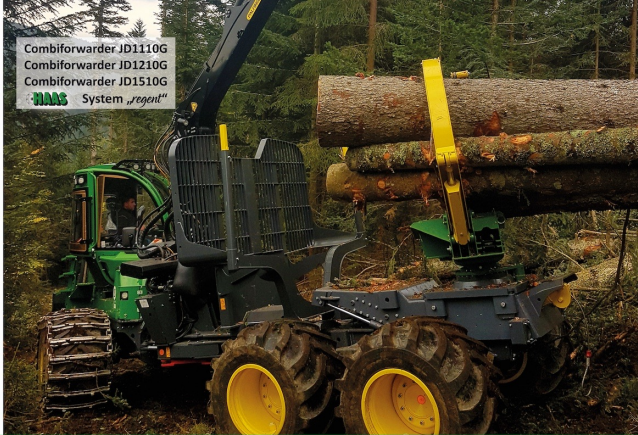
HAAS sliding rear end, headboard rear, clamping bank retracted. Shortens the rear and increases the rope entry.
