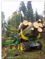
HAAS-ÖSA Clamping bank with extended movable rear for short logs.
