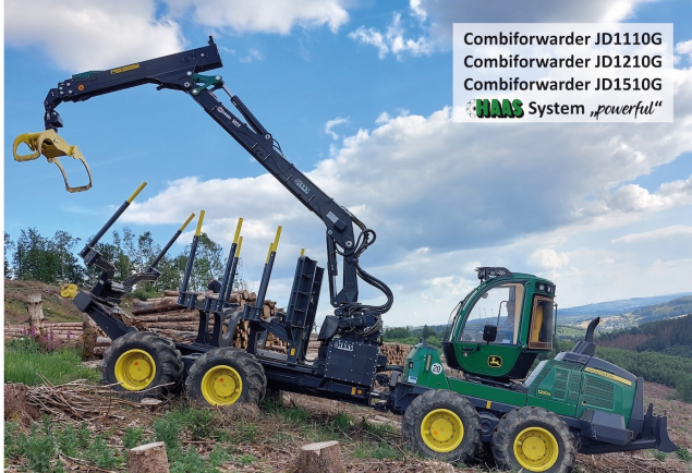
1. HAAS-OSA clamping bank for two different positions, second stake and headboard can be moved horizontally.
