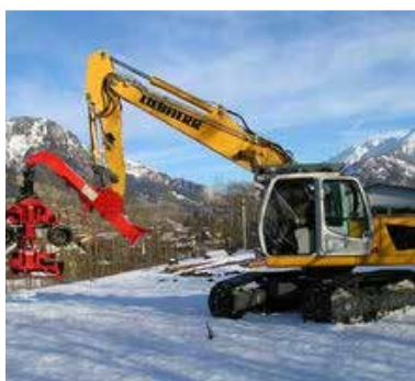
Waratah H290 Harvester Head mwith excavator foot
